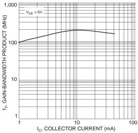
Fig. 12 Typical Gain-Bandwidth Product vs. Collector Current
