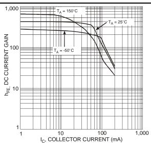
Fig. 10 Typical DC Current Gain vs. Collector Current
