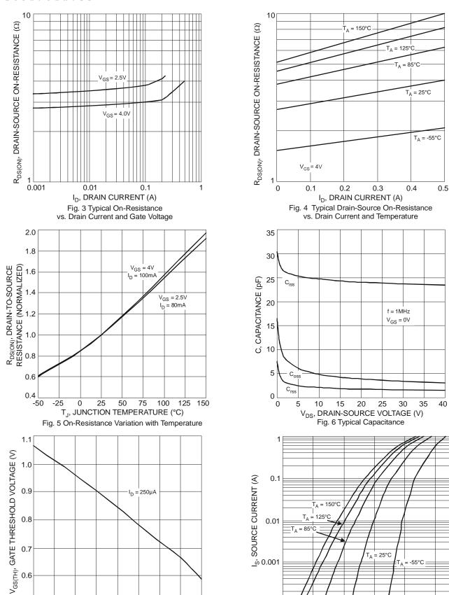
5 0 25 50 75 100 1 T<sub>A</sub>, AMBIENT TEMPERATURE (°C) Fig. 7 Gate Threshold Variation vs. Ambient Temperature
