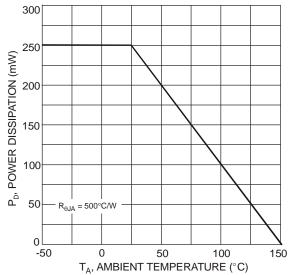
Fig. 9 Derating Curve - Total Package Power Dissipation
