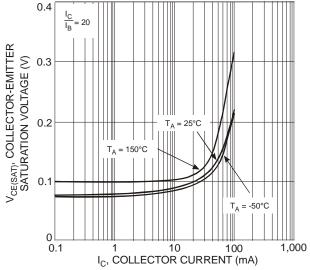
Fig. 11 Typical Collector-Emitter Saturation Voltage vs. Collector Current
